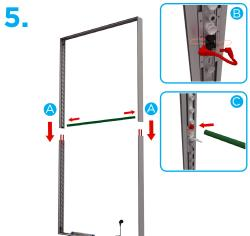
• Place the top half of the extrusion and slide onto the split connector of the bottom half extrusion. Connect LED Wire Connector to LED strips. Install Support Pole on each side of the inner frame.
