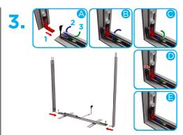
Slide side extrusions into bottom extrusion channel. Use latch to press down on the L connector. Then press down the second latch to secure. Connect LED strip cable to LED edge light connectors.
