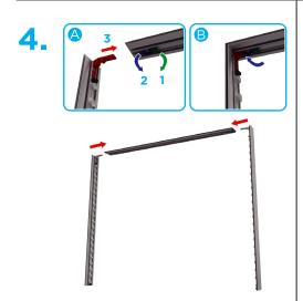
Slide side extrusions into top extrusion channel. Use latch to press down on the L connector. Then press down the second latch to secure.
