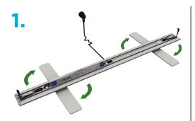
• See numbers on each extrusion piece. Match number together (e.g. 3-3). From the bottom extrusion, twist the feet.
