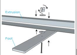
Connect the Feet to the assembled frame by locating the drill holes on the bottom Extrusion Check all extrusions if you can not immediately locate the drill holes. Feed the hardware through the **Extrusion** drill holes, tighten and attach the foot. Repeat steps for the other foot.
