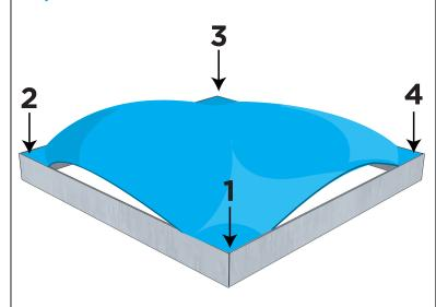
Push the silicone edge into each corner of the frame extrusions (1-4) with your thumb.
