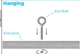
Connect the **Eye Bolt** to the assembled frame by locating the drill holes on the top Extrusion. Check all extrusions if you can not immediately locate the drill holes. Feed the Eye Bolt through the Extrusion drill holes, tighten and attach. Repeat steps for the remaining Eye Bolt(s).
