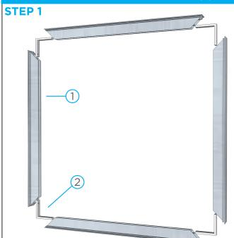
Depending on the size of the frame, form a square or rectangle by laying out the Extrusions<sup>1</sup> and the L Brackets<sup>2</sup> as illustrated.
