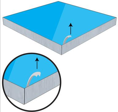
To remove the graphic pull the tab located on the graphic and gently pull the graphic from the frame, going around the perimeter.
