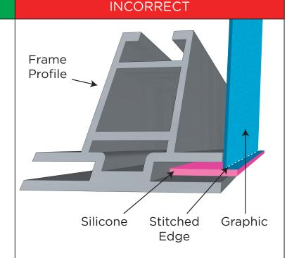
NOTE: Locate the silicone edge on the graphic which is sewn on the back perimeter. When installing the graphic be certain to insert the silicone edge correctly. The stitched edge on the silicone should be inserted first. If done correctly the silicone edge will completely fit in the graphic channel and no longer be visible once installation is complete. Continued —
