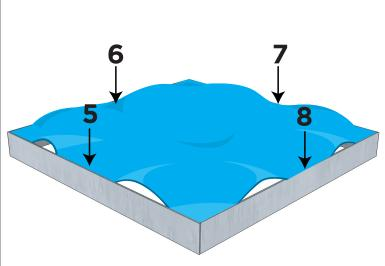
Push the silicone edge into the middle of each frame extrusions (5-8) and work your way around the perimeter of the frame until the silicone edge of the graphic is pushed in properly.
