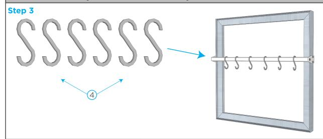
Lastly, Attach the **S-Hooks**<sup>3</sup> onto the **Dowel**<sup>5</sup>. Use the **S-Hooks**<sup>3</sup> to hang any swatches, sample, or accessory. You may want to attach the graphic to the Optium frame before you attach the **Arm Bar** for an easier graphic install.
