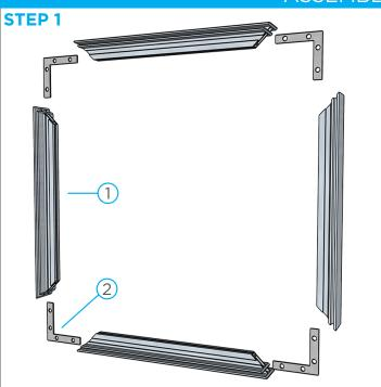
Depending on the size of the frame, form a square or rectangle by laying out the **Extrusions**<sup>1</sup> and the **Brackets**<sup>2</sup> as illustrated.
