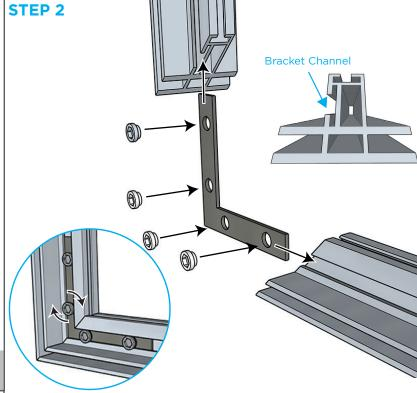
Connect all four corners by inserting the  $Brackets^2$  into the bracket channel of the  $Extrusions^1$ . Join the corners together by tightening the screws on the  $Brackets^2$ .
