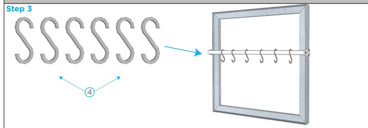
Lastly, Attach the **S-Hooks**<sup>3</sup> onto the **Dowel**<sup>5</sup>. Use the **S-Hooks**<sup>3</sup> to hang any swatches, sample, or accessory. You may want to attach the graphic to the Optium frame before you attach the **Arm Bar** for an easier graphic install.
