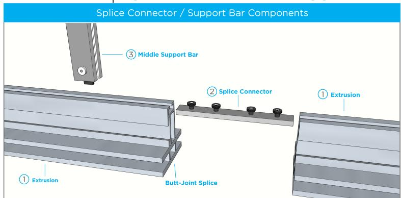
Large, oversized frames may have the Extrusions¹ spliced in half for shipping purposes. Under this circumstance you will have to use a Splice Connector<sup>2</sup> to join the Extrusions<sup>1</sup> before you begin the steps on Page 1. A Middle Support Bar<sup>3</sup> is then used to keep the Extrusions<sup>1</sup> from sagging in the middle.
