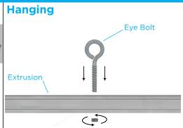
Connect the **Eye Bolt** to the assembled frame by locating the drill holes on the top **Extrusion**. Check all extrusions if you can not immediately locate the drill holes. Feed the **Eye Bolt** through the **Extrusion** drill holes, tighten and attach. Repeat steps for the remaining **Eye Bolt(s)**.
