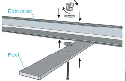
Connect the **Feet** to the assembled frame by locating the drill holes on the bottom **Extrusion**. Check all extrusions if you can not immediately locate the drill holes. Feed the hardware through the **Extrusion** drill holes, tighten and attach the foot. Repeat steps for the other foot.
