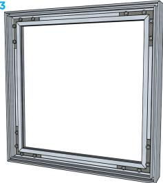
The frame is now fully assembled. The corners should be flush to each other and form a right angel. Adjust the corners if necessary.
