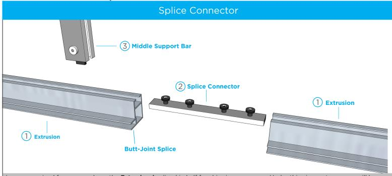
Large, oversized frames may have the **Extrusions¹** spliced in half for shipping purposes. Under this circumstance you will have to use a **Splice Connector²** to join the **Extrusions¹** before you begin the steps on **Page 1.** A **Middle Support Bar³** is then used to keep the **Extrusions¹** from sagging in the middle.
