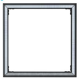
The frame is now fully assembled. The corners should be flush to each other and form a right angel. Adjust the corners if necessary.
