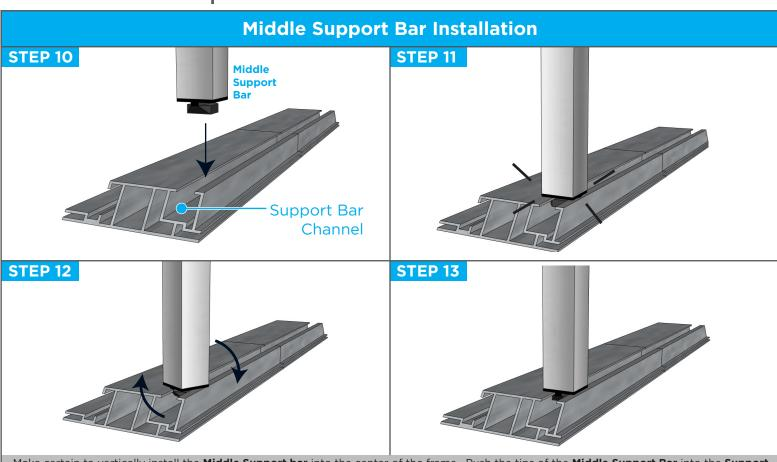
Make certain to vertically install the Middle Support bar into the center of the frame. Push the tips of the Middle Support Bar into the Support Bar Channel; then twist the Middle Support Bar 90 degrees until it is fastened to the frame. Installation of the Middle Support Bar is complete.
