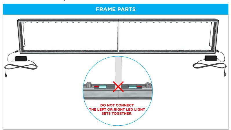
The Installation of the LED Lights is complete. You should have two separate light configurations for the Left and Right halves of the frame as shown in the illustration above. THE LEFT AND RIGHT SIDE LED LIGHTS SHOULD NOT BE CONNECTED TOGETHER. MORE THAN 6 LEDS TO A POWER ADAPTER WILL BURN IT OUT.
