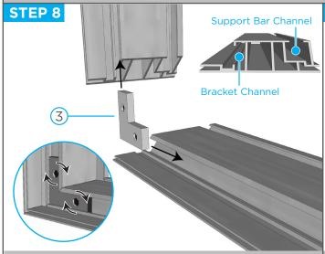
Connect all four corners by inserting the L Brackets into the "Bracket Channel" of the **Extrusions**. Join all of the corners together by tightening the screws on the L Brackets.
