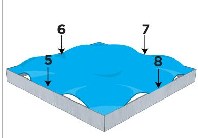
Push the silicone edge into the middle of each frame profile (5-8) and work your way around the perimeter of the frame until the silicone edge of the graphic is pushed in properly.
