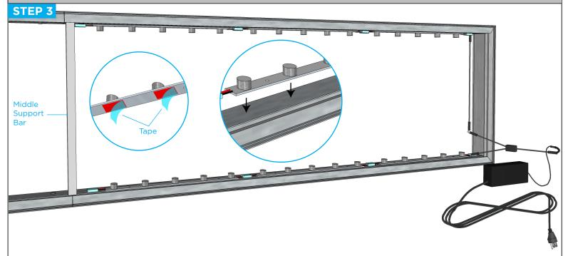
(Viewed From Back Of The Frame). On the left half of the frame attach 3 LED Lights to the bottom and 3 LED Lights to the top of the frame using the tape on the bottom of the LED Lights. Use the provided clips to attach the 5ft Extension Cable to the side of the frame. Using the remaining parts, Repeat the LED Light Assembly instructions to complete the lighting installation for the right half of the frame.
