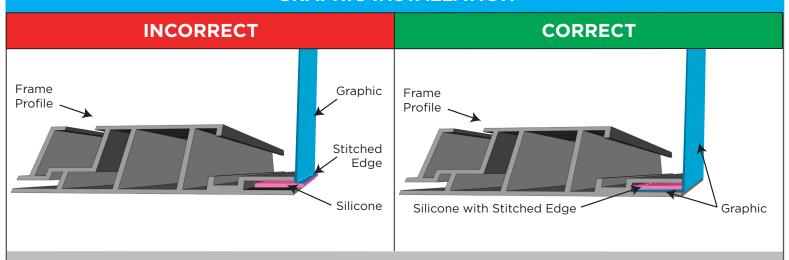
NOTE: Locate the silicone edge on the graphic which is sewn on the back perimeter. When installing the graphic be certain to insert the silicone edge correctly. The stitched edge on the silicone should be inserted first. If done correctly the silicone edge will completely fit in the graphic channel and no longer be visible once installation is complete.
