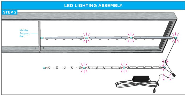
(Viewed From Back Of The Frame) Begin connecting the (x6) LED Lights, (x1) 5ft Extension Cable, (x1) Y-Splitter and (x1) Power Adapter as illustrated. Remember, DO NOT plug more than 6 LED Lights into 1 Power Adapter. Plug in the Power Adapter and test the lighting.
