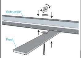
Connect the **Feet** to the assembled frame by locating the drill holes on the bottom Extrusion Check all extrusions if you can not immediately locate the drill holes. Feed the hardware through the **Extrusion** drill holes, tighten and attach the foot. Repeat steps for the other foot.
