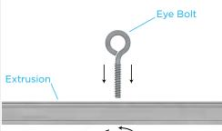
Connect the **Eye Bolt** to the assembled frame by locating the drill holes on the top **Extrusion**. Check all extrusions if you can not immediately locate the drill holes. Feed the Eye Bolt through the Extrusion drill holes, tighten and attach. Repeat steps for the remaining Eye Bolts.
