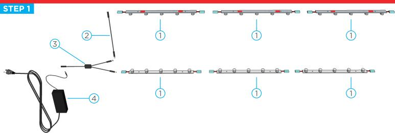
Lay out (x6) LED Lights, (x1) 5ft Extension Cable, (x1) Y-Splitter and (x1) Power Adapter as illustrated. These components will create the lighting for the left half of the frame. The remaining unused parts will be used later for the right half of the frame.
