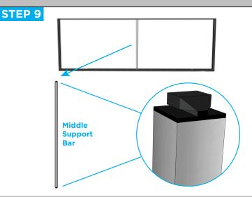
You will have to install a **Middle Support Bar** to keep the frame from sagging in the middle.
