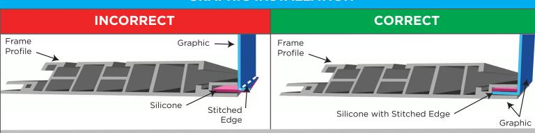
**NOTE:** Locate the silicone edge on the graphic which is sewn on the back perimeter. When installing the graphic be certain to insert the silicone edge correctly. The stitched edge on the silicone should be inserted first. If done correctly the silicone edge will completely fit in the graphic channel and no longer be visible once installation is complete.
