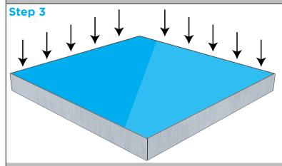
If necessary; Go around the perimeter again to ensure the silicone edge is secure and hidden in the frame profile. The graphic should be smooth and taut.
