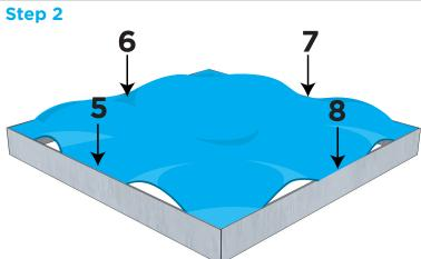
Push the silicone edge into the middle of each frame profile (5-8) and work your way around the perimeter of the frame until the silicone edge of the graphic is pushed in properly.
