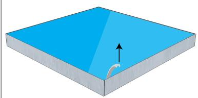
To remove the graphic pull the tab located on the graphic and gently pull the graphic from the frame, going around the perimeter.
