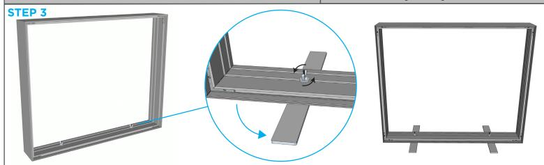
The frame is now fully assembled. The corners should be flush to each other and form a right angel. Adjust the corners if necessary. Next, turn the foot plates on the bottom of the frame outward, 90 degrees, and tighten the foot plate wing nuts. Now you can stand the frame upright.
