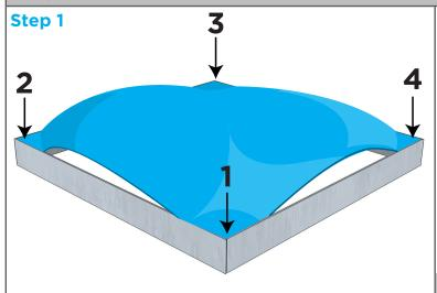
Push the silicone edge into each corner of the frame profile (1-4) with your thumb.
