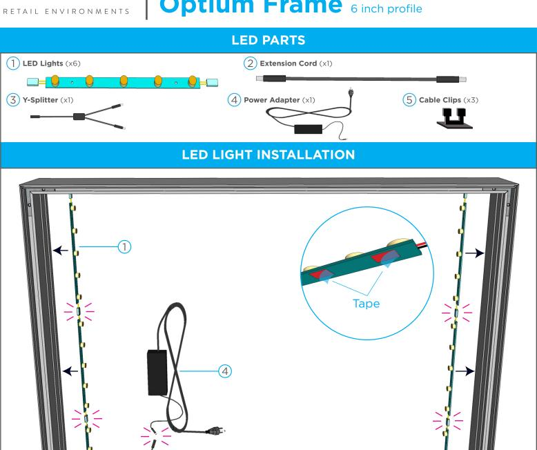
Using the tape on the bottom of the LED Lights<sup>1</sup>, evenly distribute and attach the LED Lights<sup>1</sup> on center, to the sides of the frame. Begin connecting the LED Lights¹, Extension Cable², Y-Splitter³ and Power Adapter⁴ as illustrated. Use the Cable Clips⁵ to attach the Extension Cable<sup>2</sup> to the frame. The installation of the LED Lights is complete. Plug in the Power Adapter⁴ to an outlet and test.
