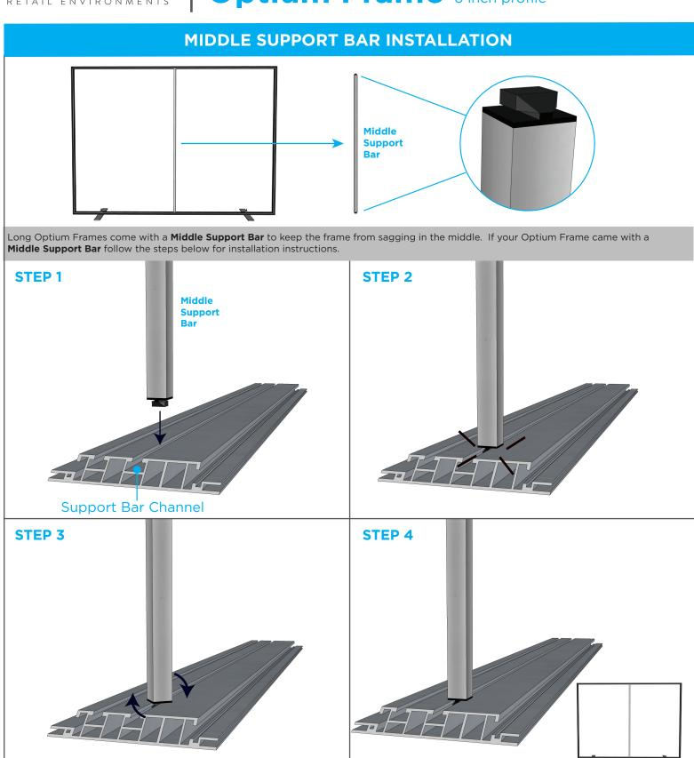
Make certain to vertically install the **Middle Support bar** into the center of the frame. Push the tips of the **Middle Support Bar** into the **Support Bar Channel**, then twist the **Middle Support Bar** 90 degrees until it is fastened to the frame. Installation of the **Middle Support Bar** is complete.
