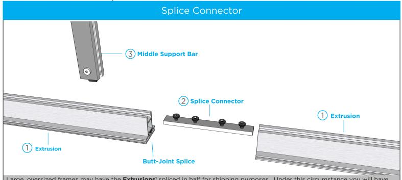
Large, oversized frames may have the Extrusions spliced in half for shipping purposes. Under this circumstance you will have to use a Splice Connector<sup>2</sup> to join the Extrusions<sup>1</sup> before you begin the steps on Page 1. A Middle Support Bar<sup>3</sup> is then used to keep the Extrusions<sup>1</sup> from sagging in the middle.
