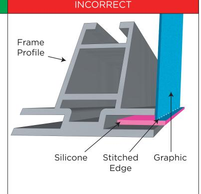
NOTE: Locate the silicone edge on the graphic which is sewn on the back perimeter. When installing the graphic be certain to insert the silicone edge correctly. The stitched edge on the silicone should be inserted first. If done correctly the silicone edge will completely fit in the graphic channel and no longer be visible once installation is complete. Continued -
