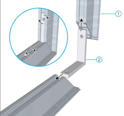
Connect all four corners by inserting the **L Brackets**<sup>2</sup> into the bracket channel of the **Extrusions**<sup>1</sup>. Join the corners together by tightening the screws on the L Brackets<sup>2</sup>.
