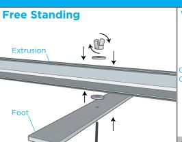
Connect the **Feet** to the assembled frame by locating the drill holes on the bottom Extrusion Check all extrusions if you can not immediately locate the drill holes. Feed the hardware through the Extrusion drill holes, tighten and attach the foot. Repeat steps for the other foot.
