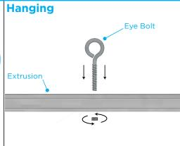
Connect the **Eye Bolt** to the assembled frame by locating the drill holes on the top **Extrusion**. Check all extrusions if you can not immediately locate the drill holes. Feed the **Eye Bolt** through the **Extrusion** drill holes, tighten and attach. Repeat steps for the remaining **Eye Bolt(s)**.
