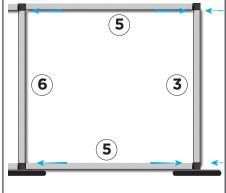
Repeat Step 2 for the second sidebar with connectors and silver bars. A rubber mallet or hammer and wood block may be needed to tap the tube completely onto the connector.
