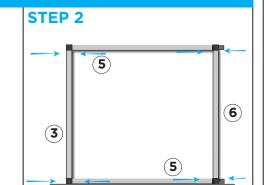
Insert connector bolts through base from bottom, and connect to threaded bottom bar corners using the supplied allen wrench. Repeat this step with the outside bases.
