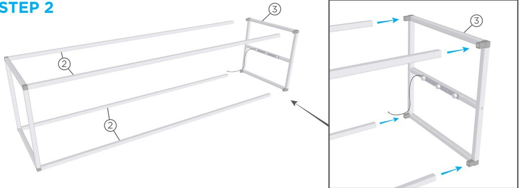
Insert the other end of the four Side Bars into the connectors of the LED Frame Base.
