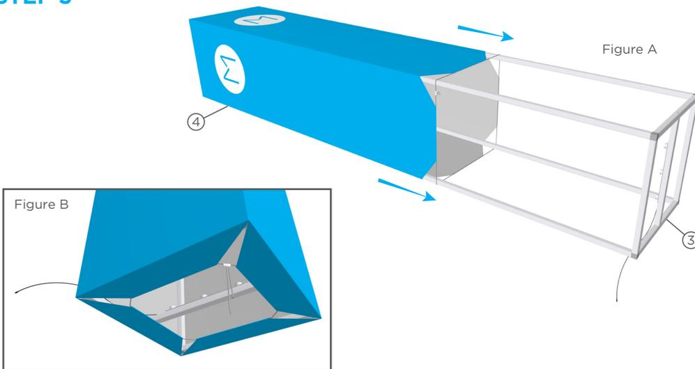
Pull the graphic over the Frame Top, pulling it toward the LED Frame Base until it is taut at the bottom of the assembled frame (Figure A). Secure the graphic by adjusting the drawstring at the base of the graphic and thread the end of the LED power cord through the slit at the base of the graphic (Figure B).
