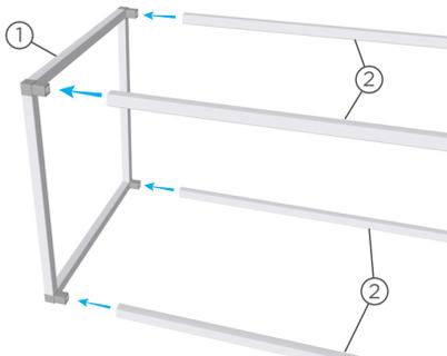
Insert a Side Bar into each of the four connectors of the Frame Top.
